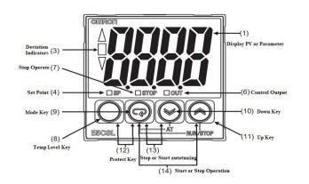
(1) Display the Process Value (PV), parameter, set point and parameter setting
